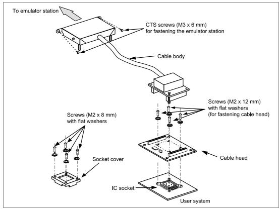
Figure 1 HS2378ECH61H User System Interface Cable
